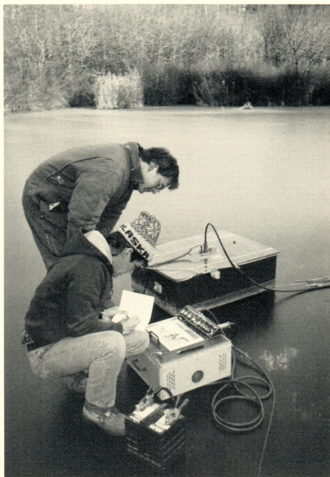
Ground Penetrating Radar Survey across a frozen lake.
