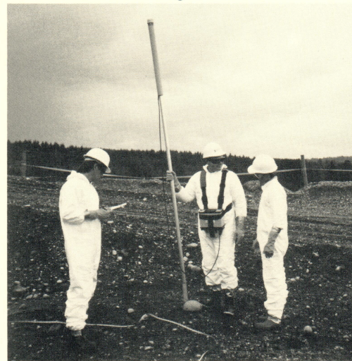
Magnetometer Survey at a hazardous waste site in Washington.
