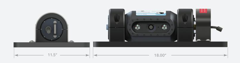
**Depth Rating** Aluminum: 1000m Viewport Sapphire Glass 11.5" wide x 18" long x 5.25" tall **Dimensions** Weight In air 18.8 lbs; in water 9.5 lbs 1080p @ 30FPS or 720p @ 30-60FPS Camera Adj. white balance & exposure 120° FOV in air 128GB solid state memory Optional time stamp & loop recording Electrical 14.4VDC 192Wh nominal 3A charge current SUBCONN MCBH 8M Connector
